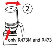
To make the adjustment the first step is the complete opening of the mechanical memory with the screwdriver part of the key R558. Then with the hexagonal part of the same key R558 you must open the lockshield until the required value. After this you must close the mechanical memory with the screwdriver part of the key R558.
